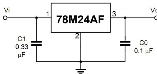
Note : Bypass capacitors are recommended for optimum stability and transient response and
