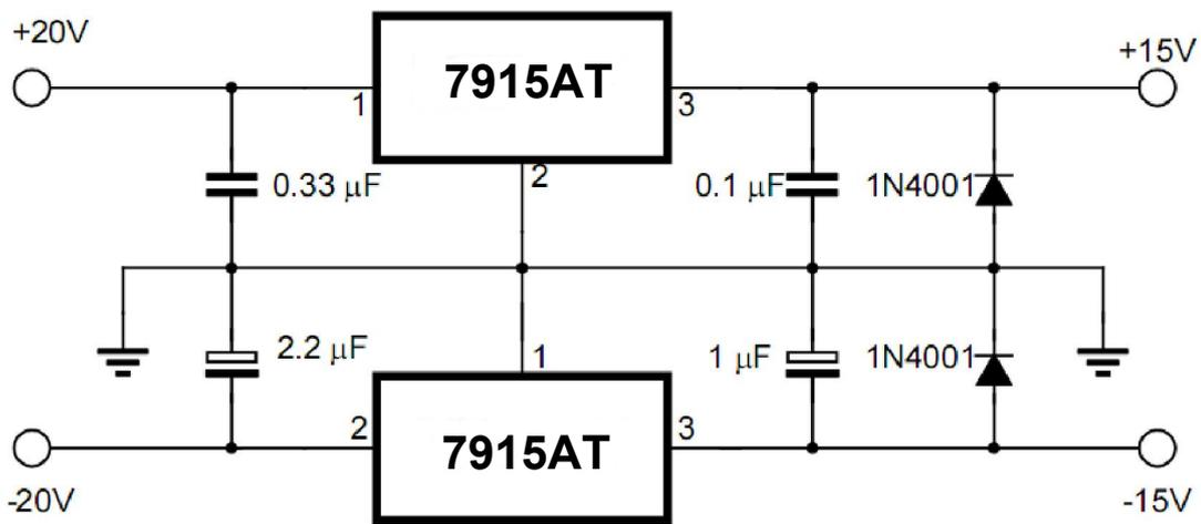
Figure 2. Split power supply ( $\pm 15\text{ V}$ ,  $-1.5\text{ A}$ )
